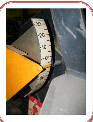
This is to measure the angle of the load on the forklift.
