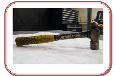
This hammer has a grip on the handle. The grip is yellow and is made out of rubber. It will help you to hold onto the hammer so it does not slip out of your hand.
