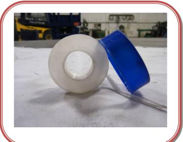
This is a roll of Teflon tape. It is white and you would use it to seal pipe connections. It is thin and stretchy.
