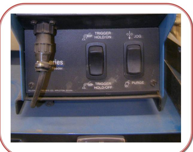
Here you can see the switch for the Trigger Hold, on and off. You can also see the switch to Jog or Purge.
