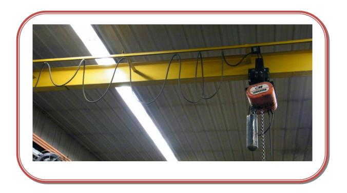
In this picture you can see how the cable moves along the track.
