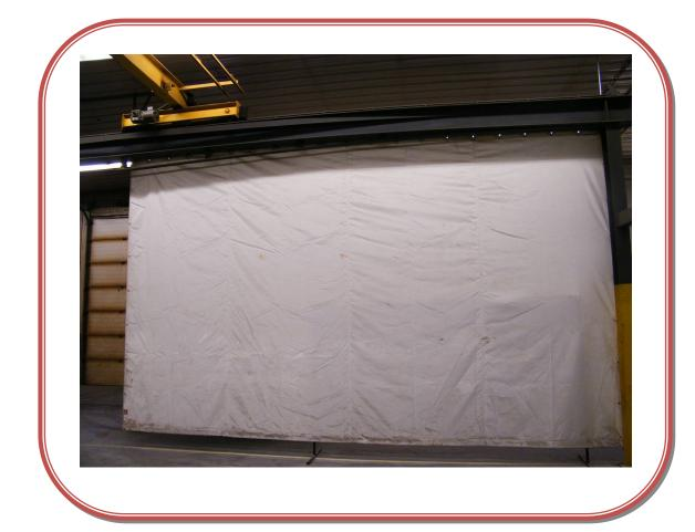
This is a welding curtain. It stops the sparks that the welder makes from spreading.
