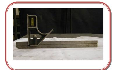
The square level has measurement in inches. You can slide the level by turning the knob and moving it along the ruler.
