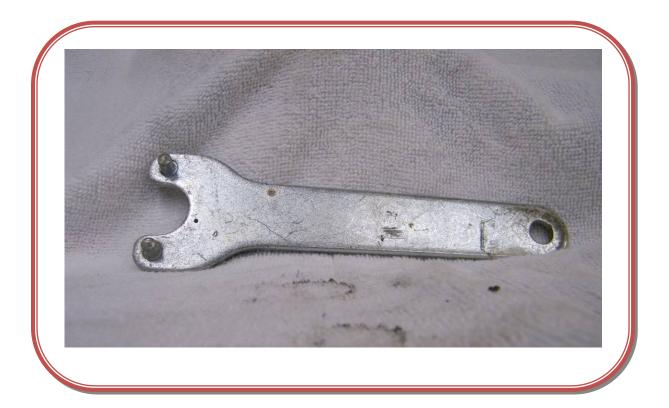
This is a tool needed to tighten and loosen the wheel on the grinder.
