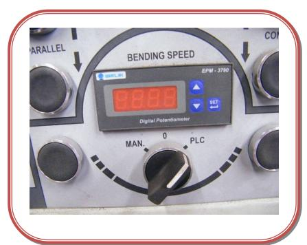
This is the control to set the speed of the rollers or the bending speed.
