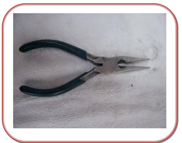
This is a pair of needle nose pliers. They can get into very small spaces. They can also cut wire.
