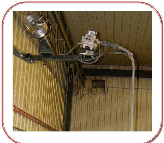
In this picture you can see the roll of welding wire being fed into the Mig welder.
