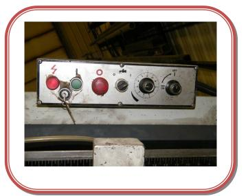
Can you see the buttons and switches that control the machine? You also need to have a key to start this machine.
