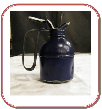
This is an oil can. It helps you to put a drop of oil in a small space.
