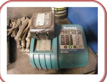
This is where the battery is placed when it needs to be recharged. The light is green so that means that the battery is ready to use.
