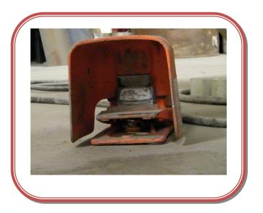
Can you see the strong spring inside the foot pedal that must be pushed down with your foot to allow power to go to the Shear?
