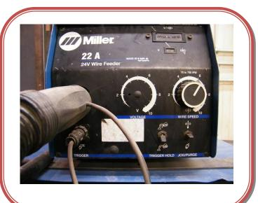
Can you find the controls for the Voltage, the Wire Speed, and the Trigger?
