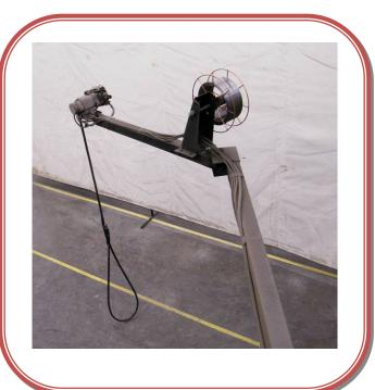
In this picture you can see the welding wire and the welder tip.
