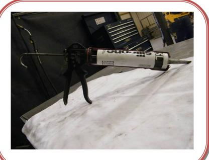
This is a tube of silicone. Silicone is used to seal edges together so that no water can get in.
