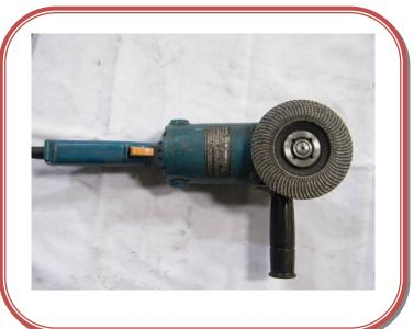
The trigger on the hand grinder is orange. It will turn the power on or off.
