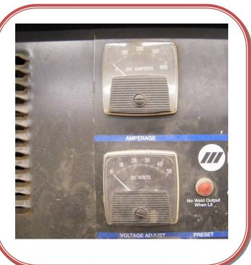
These are the controls for the Amps and for the Voltage.
