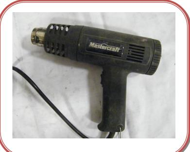
This is a heat gun. It can be used to make things soft and pliable.
