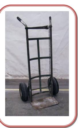
This dolly has a tarp strap and a chain. These will keep the load from shifting or falling off.
